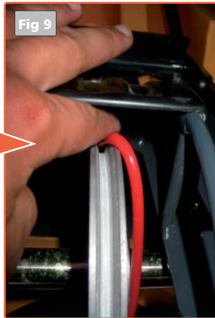
Roll the belt under the large 'V' pulley and hold near the top. (fig 8 and 9)
