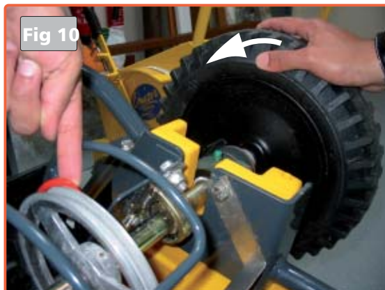
While holding the belt turn the drive wheel to roll the belt into the groove. Ensure that the belt is seated in the pulley. (fig 10 and 11) Check the orientation of the belt with fig 2 and 3.
