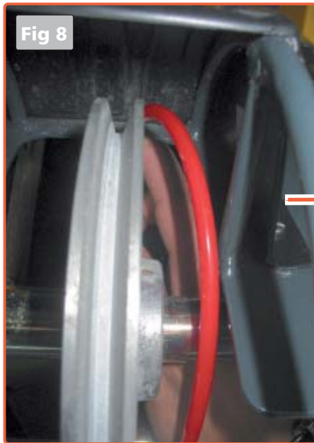
Roll the belt under the large 'V' pulley and hold near the top. (fig 8 and 9)
